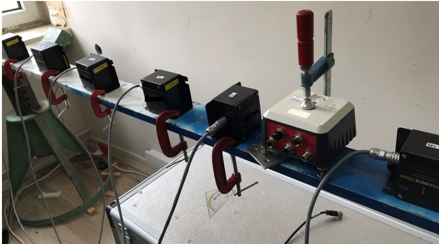
Figure 3.3 : Sensor locations and simply supported beam
